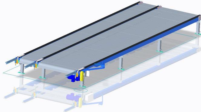
Transport and buffer table for building elements in horizontal position. Equipped with flat chain tracks and frequency-controlled operation for efficient and gentle transport. Integrates into the robot cell.
