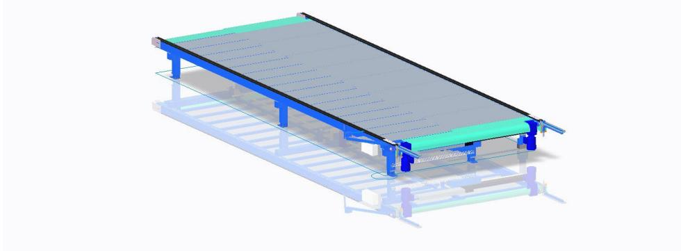
Working table to safely transport and process the wall element. Chain conveyors transport the wall element. The motorized width adjustment is adjusted to accommodate incoming wall elements.
