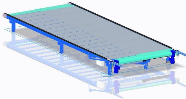
Working table to safely transport and process the wall element. Chain conveyors transports the wall element into the station. Motorized width adjustment in two positions is automatically adjusted for adaptation of incoming wall elements.
