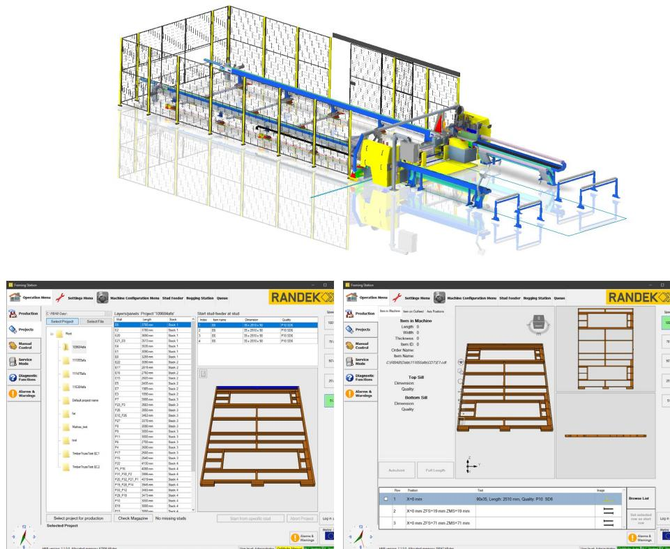
Framing station FM3000 for the manufacturing prefabricated wall frameworks. The machine requires CAD / CAM connection. Visualization of the element on the HMI screen makes it easy to follow the construction process.
