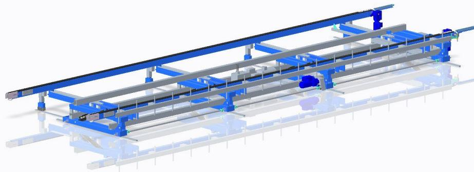
Randek's upraiser table is an efficient and flexible tool when upraising the building elements. Equipped with flat-chain conveyors for efficient and gentle transport. Upraising function with hydraulic cylinders for safe and precise handling of the building element. Movable sideways.
