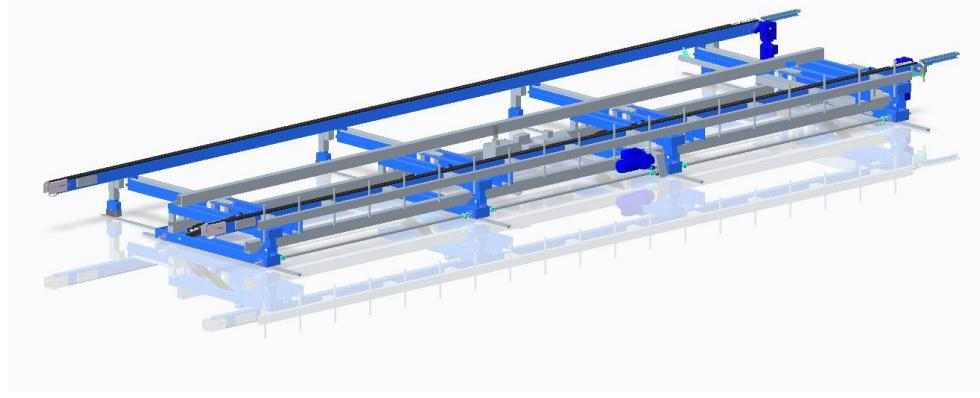
Randek's work and upraiser table is an efficient and flexible tool for upraising and machining the building elements. Equipped with flat-chain conveyors for efficient and gentle transport. The motorized width adjustment is adjusted to accommodate incoming wall elements. Upraising function with hydraulic cylinders for safe and precise handling of the building element. Movable sideways to raise up before discharge of finished element.
