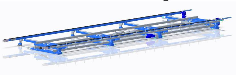
Randek's working and receiver table is an efficient and flexible machine when turning and working on the building element. Turning function with hydraulic cylinders for safe and precise handling of the building element. The motorized width adjustment is adjusted to accommodate incoming wall elements. Movable sideways to meet the associated upraising table.
