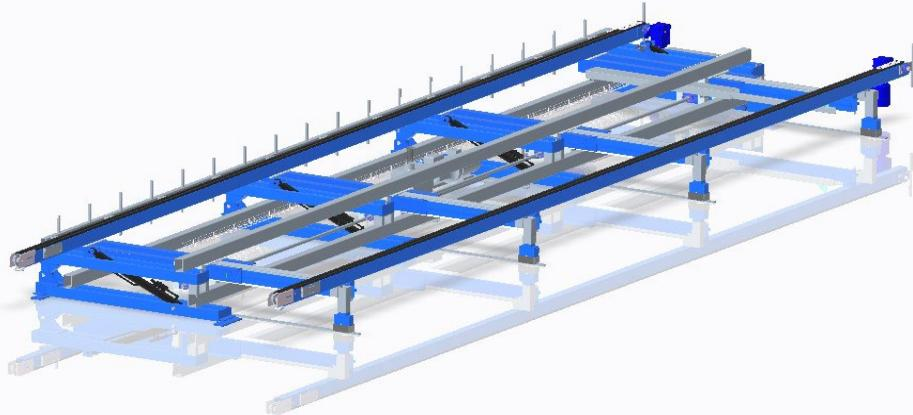
Randeks upraiser table is an efficient and flexible machine for turning or raising the wall elements. Equipped with flat-chain conveyors for efficient and gentle transport. Upraising function with hydraulic cylinders for safe and accurate raising of the wall element.
