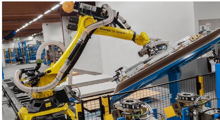
Both robots have a set of tools with associated tool racks. When the tools' magazines start to run out, the system notifies the operators that they are ready to refill. It is possible to load a magazine in the tool rack from a safe position while the robots are working, which enables high availability.
