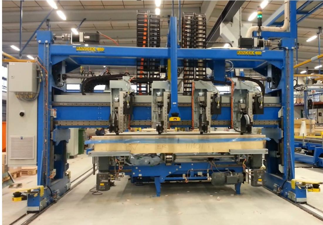
Randek's multifunction bridge, NB3000, is designed to automatically fasten and process sheet material on a framework. Equipped with up to four tool carts for fastening tools, which provides great flexibility for different tool configurations. The portal can also be provided with several different options for additional functions.
