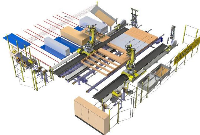
Randek's ZeroLabor robot system is a fully automatic system for handling and processing building elements. The system is flexible and can be configured according to the buyer's needs. The system is easily integrated into new production lines and existing production lines but can also be used as a stand-alone unit. The system can handle various forms of building elements such as walls, floors and ceilings.
