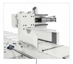
**Rapid loading of the timber** into the machine, thanks to the automatic loading system.
