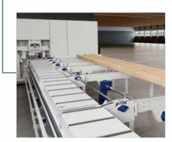
**Possibility of positioning a series of beams** by means of the motorised chain loading system with buffer.
