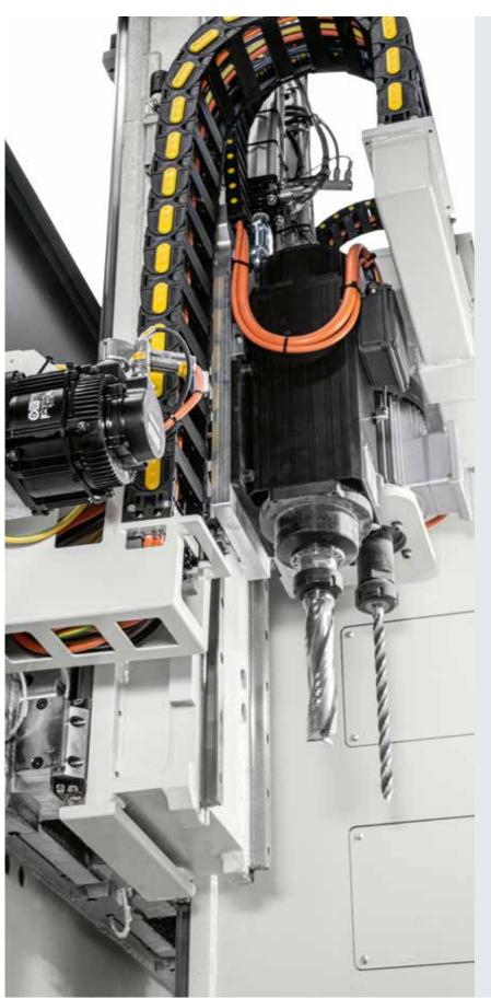
The 3-axis vertical drilling and routing units, compatible with drill bits and end mills, are dedicated to the execution of through or blind machining operations on the workpiece upper face.
