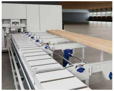
Consisting of a series of supports with variable spacing, it allows the loading of timber up to 16 metres long, 450 mm wide and 240 mm thick.
