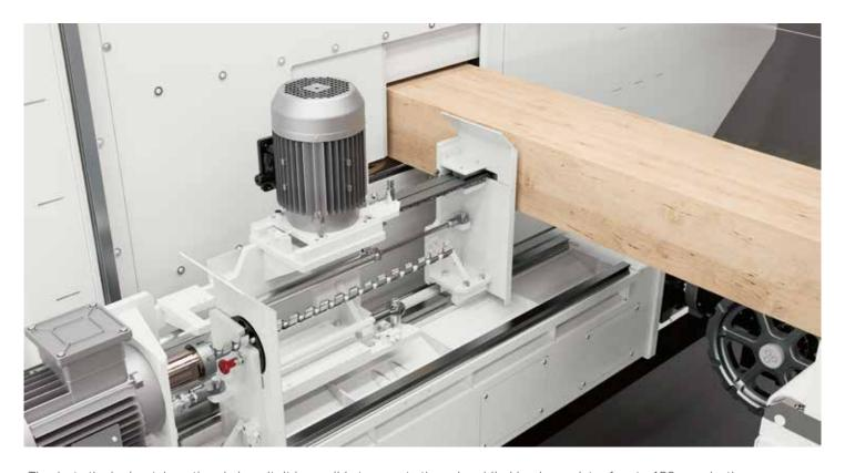
Thanks to the horizontal mortise chain unit, it is possible to execute through or blind hardware slots of up to 450 mm depth.
