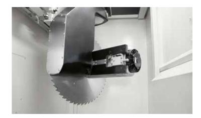
Possibility of executing markings on the 4 faces of the workpiece by means of marking devices assembled respectively on the edge of the saw blade unit and the revolver unit.
