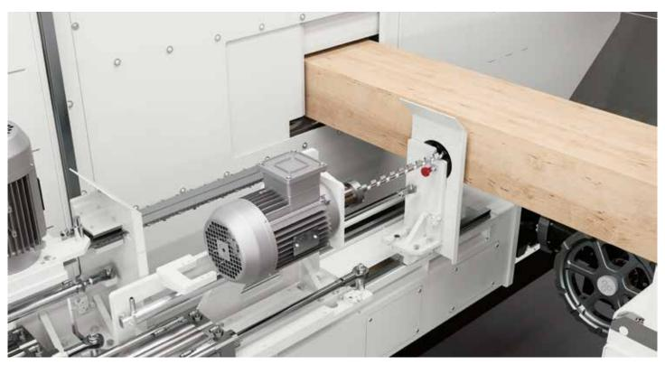
The horizontal drilling unit, positioned on the same crossbeam as the revolver unit, allows the execution of deep holes up to 450 mm from the workpiece front face. The operating unit includes a drill guide system in order to guarantee machining accuracy.
