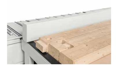
A mechanical pusher pushes the element onto the storage buffer, composed of fixed supports arranged at variable spacing. Their inclination and the presence of idle rollers allow rapid retrieval of the elements.
