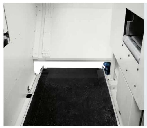
A motorised belt carries shavings and scraps outside the cabin. This system is also useful in the case of the "waste reduction function".
