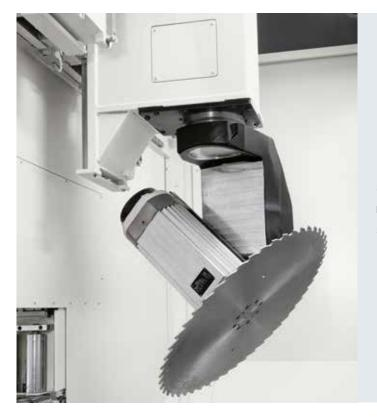
5-axis operating unit dedicated to the use of a saw blade of maximum diameter 760 mm to carry out cutting operations on the 5 faces of the element.
