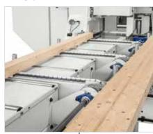
Retractable rear mechanical stops for referencing the timber at the end of the loading phase and ensuring high precision.
