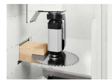
The most common operations that can be performed with the saw blade unit are straight and inclined cuts, slots for hardware, slopes and notches.
