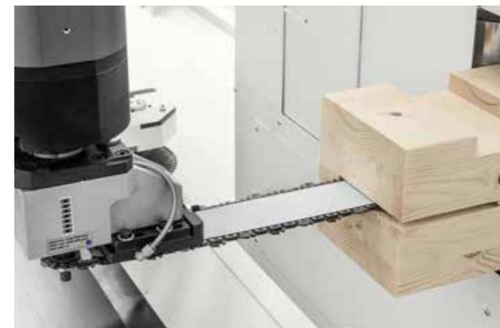
Execution of slots of 8,10,12 mm thickness.
