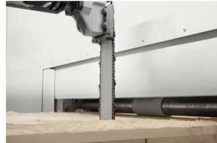
Rapid movements within the material. Chain thickness 7 mm.
