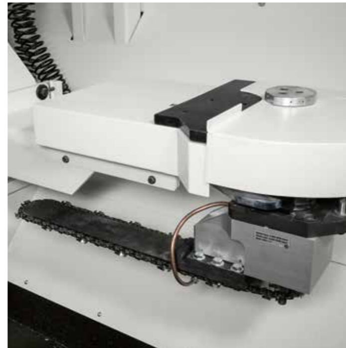
Lower position dedicated to the mortise chain aggregate or tools of up to 15 kg weight
